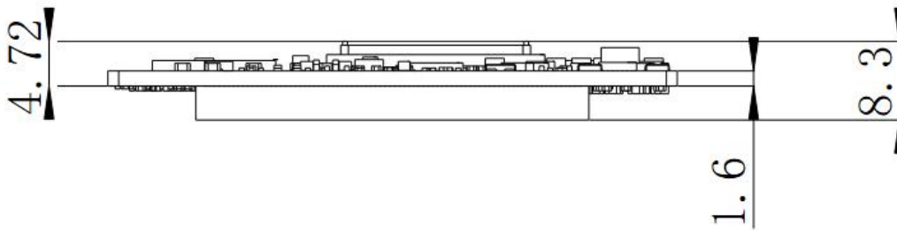
Dimensions of MYC-CZU3EG-V3 (Side-view, without heatsink)
