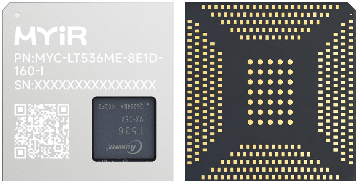
MYC-LT536 System-On-Module Top-view and Bottom-view
