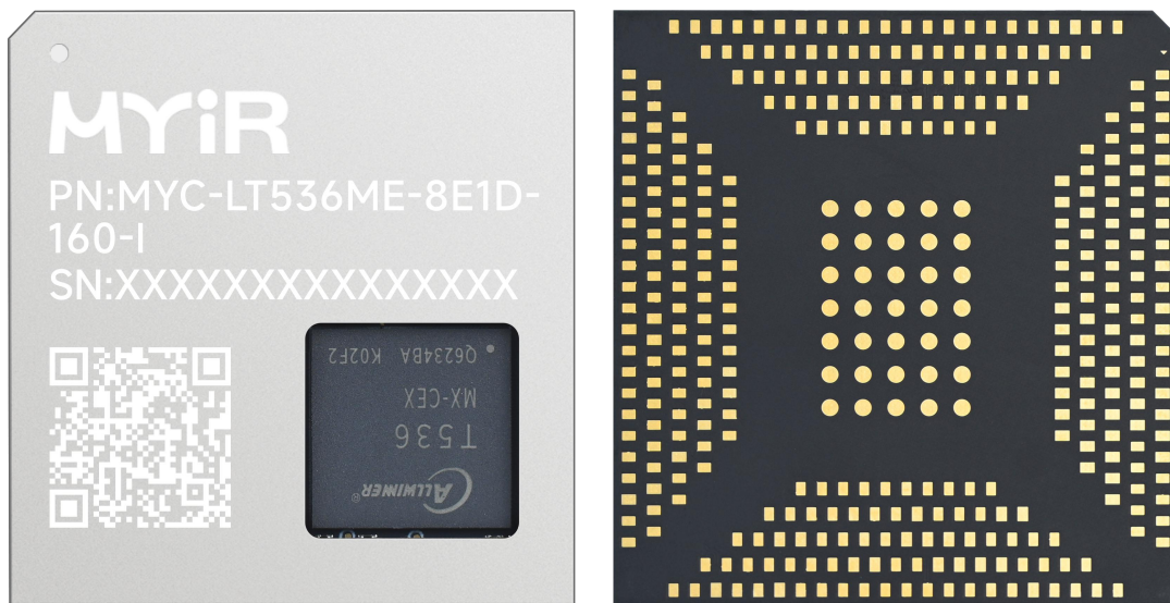
MYC-LT536 System-On-Module (Top-view and Bottom-view)
