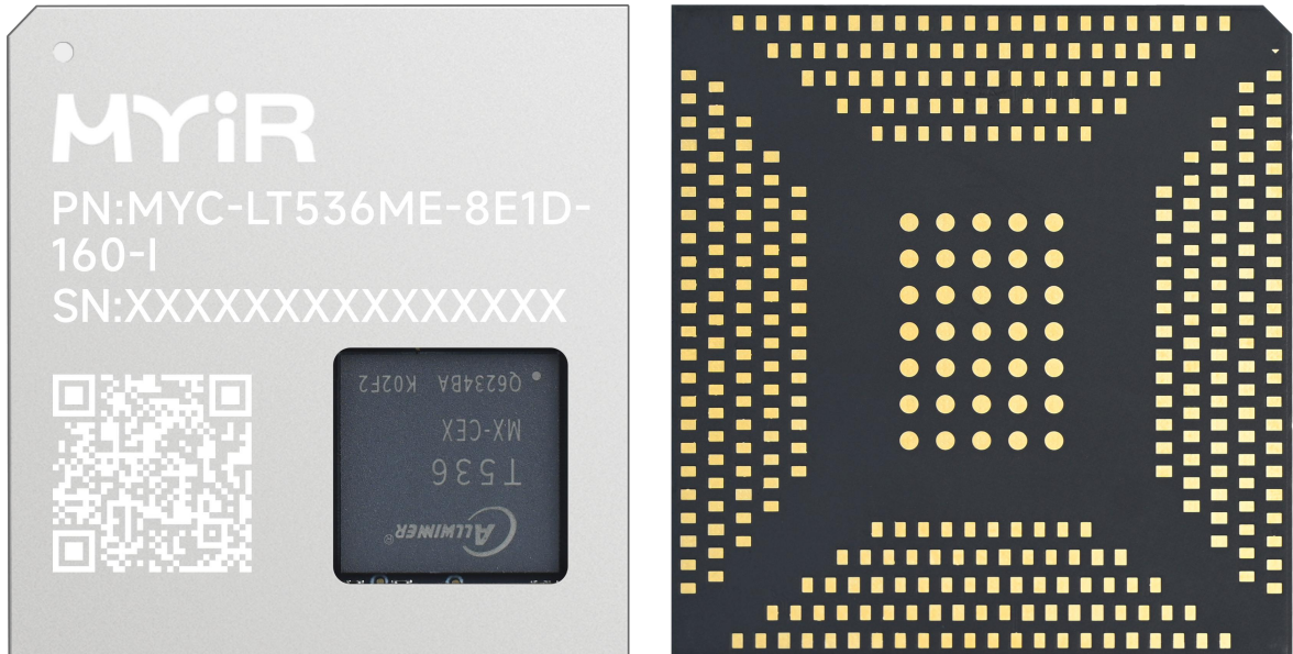
MYC-LT536 System-On-Module Top-view and Bottom-view
